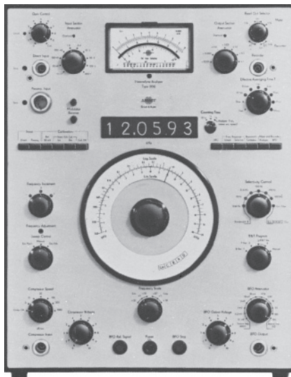
FIGURE 10.25 Heterodyne analyzer. (Brüel and Kjaer Sound and Vibration Measurement A/S.)
