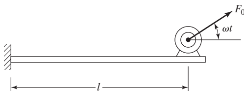
FIGURE 3.65 Unbalance in the motor supported on cantilever beam.
